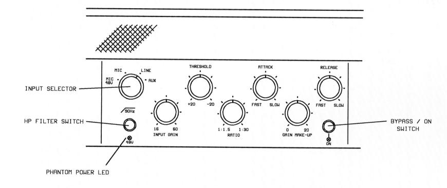
FIG.2: COMPRESSOR CONTROLS
