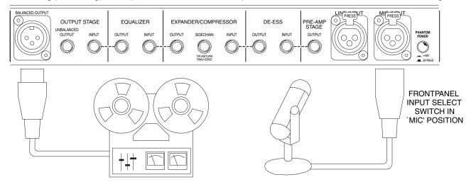
528E into a console or system having only microphone level inputs. However workable, the ultimate performance of the 528E will be limited by the performance of your system's existing microphone preamps. If you can find a way to bypass the existing microphone preamps in your system, do so. It'll be worth the trouble.
