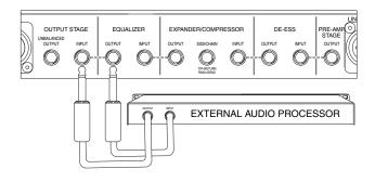
An insert or series processor is one that is inserted in series with the signal to be modified. Generally speaking, series processors have a wet-dry mix control, however compressors, expanders, gates, equalizers, as well as the 528E, are all series processors that don't.
