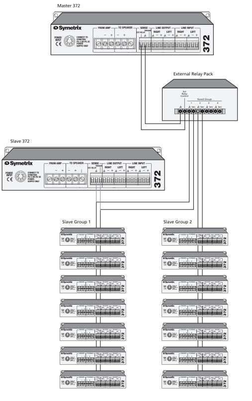
Connect a cable from EXT RELAY and Ground terminals of the master unit to the External Relay control and Ground terminals on the rear panel of the external relay.
