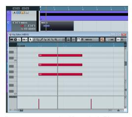
If you enter a transpose value of 7, your chord will be transposed by seven semitones upwards. In this example, this would be G3/B3/D4.
