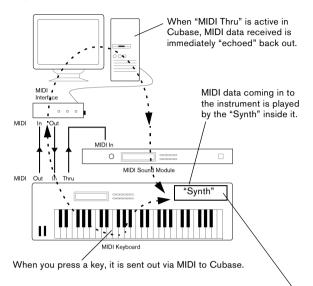
When Local Control is turned on in the instrument, the keys you press will be played by the "Synth" inside the instrument. When Local Control is turned off, this connection is cut off.
