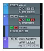
The track list showing a MIDI track, an audio track with an automation track, and a VST instrument track
