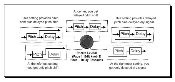
Behavior of **Effects LvI/Bal** in the cascade programs. Several points from the knob's continuous range are illustrated here, using Pitch-Delay as an example.
