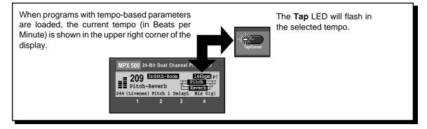
To set the tempo from the front panel, simply press the **Tap** button (or a connected footswitch) twice in time with the music. That's your tempo. No more dialing up what "could be" the delay time in milliseconds — just tap twice — the MPX 500 will figure out the time for you. When you want to change tempo, just tap twice again in the new rhythm.
