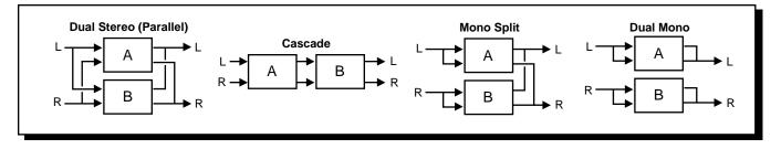
Generally, the **Effects LvI/Bal** parameter (Page 1, Edit knob 3) controls the balance of the two effects in each dual program. In the cascade variations, rather than simply controlling balance, the knob varies the amount of the first effect or dry signal which is fed into the second effect.
