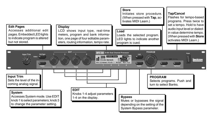
\* The level indicators are at their minimum size when the incoming signal is low (more than 30dB below full scale). The highest level indicators are highlighted when the signal approaches full scale.
