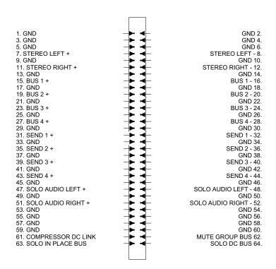
7600 BUS CONNECTOR PINOUT
