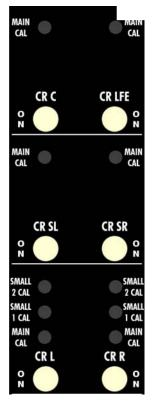
The 268B Monitor Output section supports one set of main 5.1 monitors and two sets of stereo monitors. The Monitor Output section provides on/off switching and calibration for a 5.1 (Left, Right, Center, Left Surround, Right Surround, and LFE) main monitor system (MAIN) and the two stereo nearfield monitor systems (SMALL 1 and 2). The Monitor Output section has the following features:
