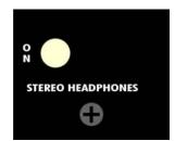
ON: On/off switch for the Stereo Headphone Amplifier
