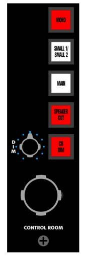
MONO: Sums the Left and Right Control Room Monitor output to mono.
