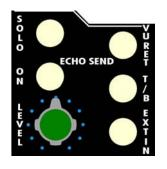
The E1608 ECHO SEND section primarily functions as an echo send master. It can also provide grouping functions when used with the echo sends, external inputs, and the Echo Return section.
