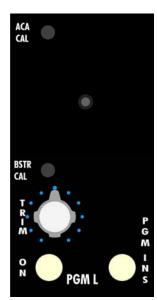
$\underline{ACA\ CAL\ (trim-pot)}$ : The trim-pot calibrates the output of the Active Combining Amplifier
