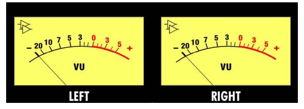
The large LEFT and RIGHT Meters display the stereo Program Master Output (post the Master Fader).
