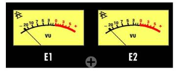
The E1 – E8 Meters display the output of the eight Echo/Auxiliary Send Masters (post the Echo Send Master).
