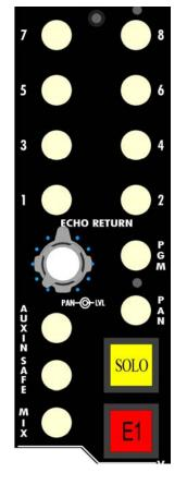
The E1608 ECHO RETURN section is an independent audio channel with multiple input options, complete level, muting, and panning controls, full solo capabilities, and full routing to the Program and Summing Buses. Some possible Echo Return applications include:
