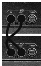
Figure 3-3. Connecting Two 1788A-R's for Cloning
